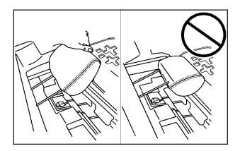
The third row seat head rests can be removed from the seatback. To do this, press the button, located on the top of the seatback, and pull them out from the seatback. Store the head rest, front side facing up, in the compartment behind the third row, by inserting the head rest posts into the slots in the storage area.
